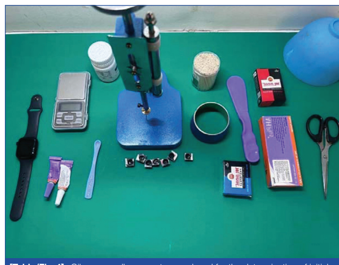
[Table/Fig-4]: Gilmore needle apparatus employed for the determination of initial and final setting times of the experimental sealers.
